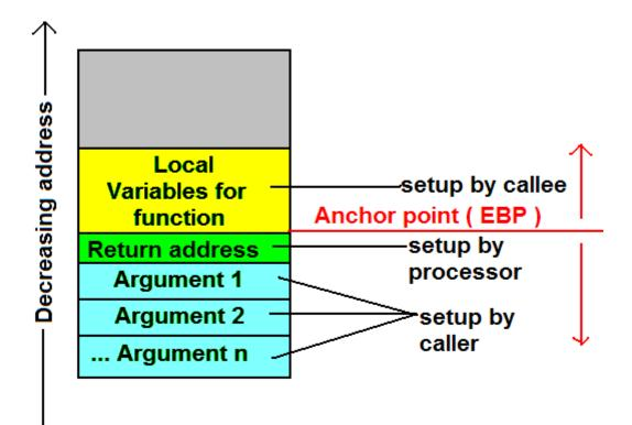
When a function is called, parameters are placed on the stack in order.
