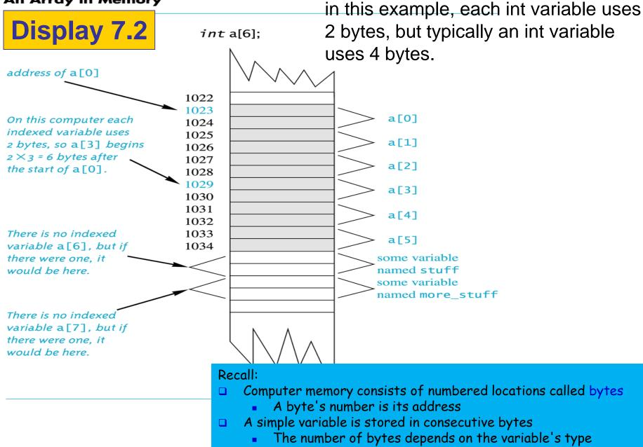
A variable's address is the address of its first byte
