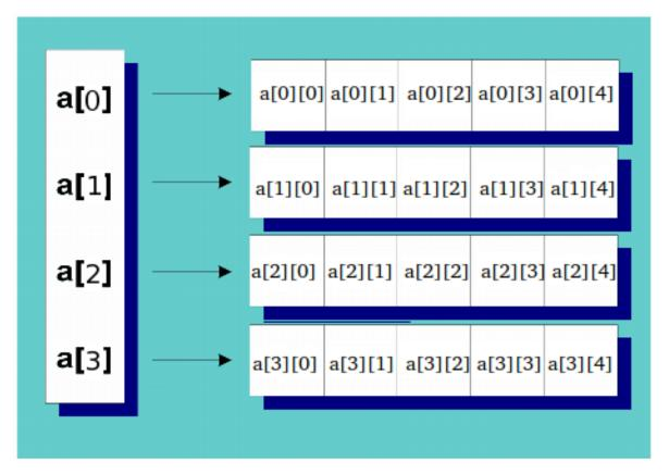
A two dimensional array is really an array of pointers to arrays
