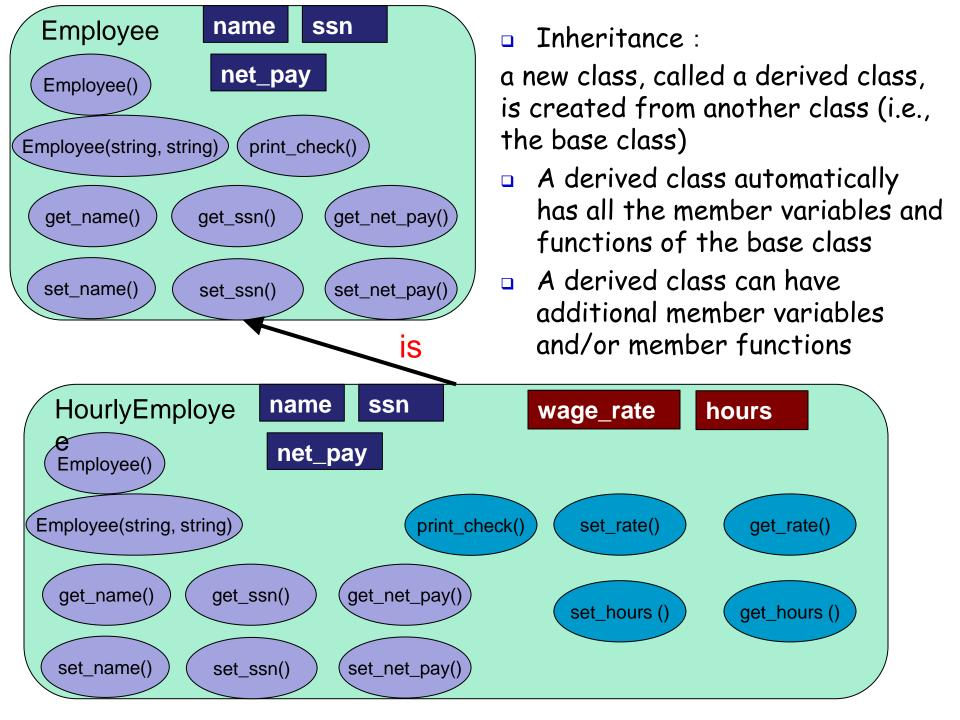
A derived class automatically has all the member variables and functions of the base class.
