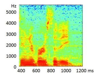
The final sound "ee" consists of the formants F1: 500 Hz and F2 2200Hz.
