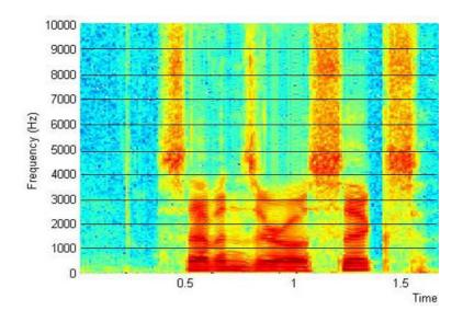
Identify the time intervals for at least three times the 's' or 'ch' sound occurs in the "spectrogram" above (plotting frequency vs time).
