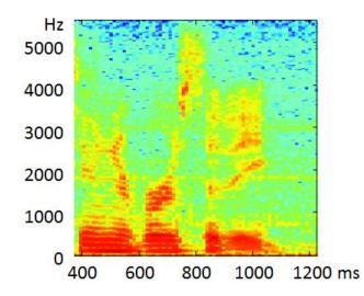
The final sound "ee" consists of the formants F1: 500 Hz and F2 2200Hz.
